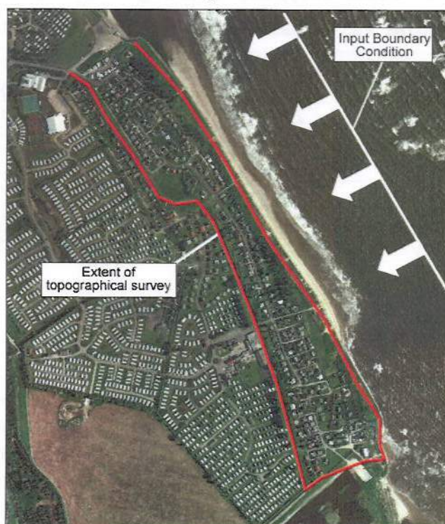
Figure 12 Model boundary conditions and crest survey
