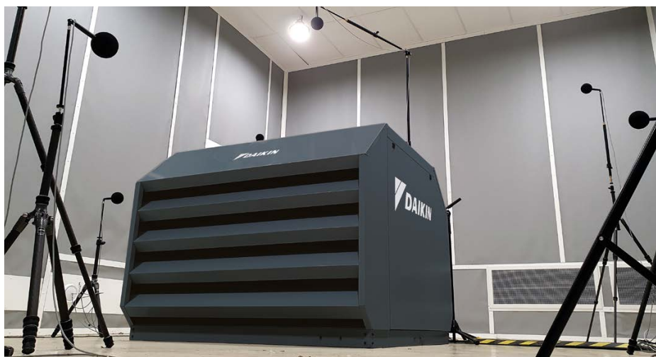
Sound power level measurement in acoustic chamber
