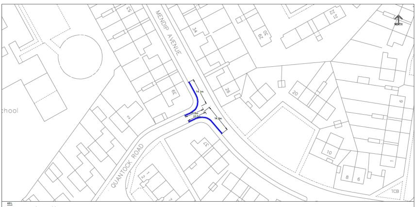
Proposed NWAAT restrictions (Double Yellow Lines) TSRGD 1018.1 (100mm wide, 100mm spacing)
