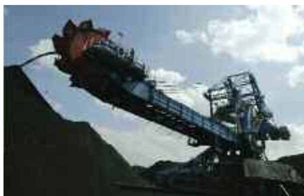
A stacker-reclaimer storing coal at the Port. Mechanised conveyor belts are used to move the material
