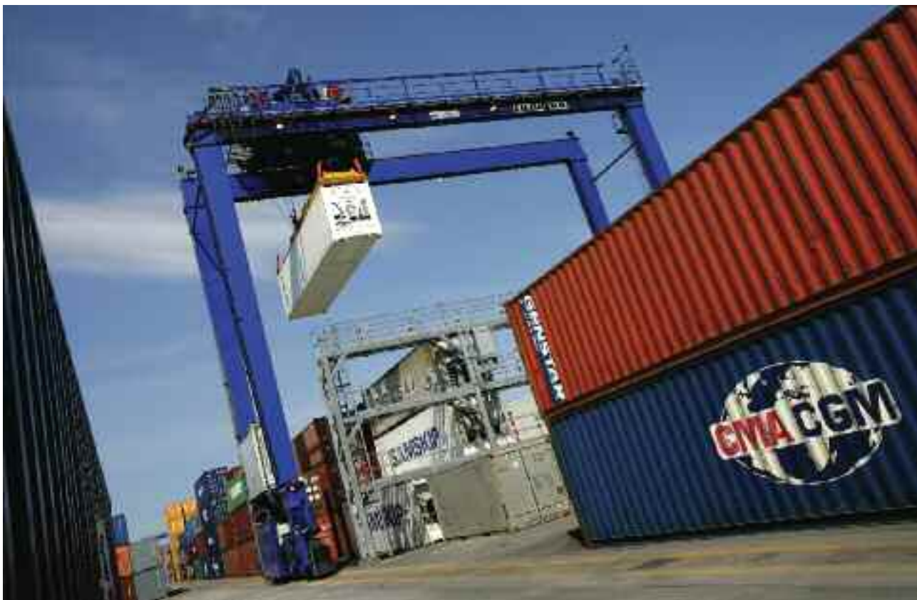
Immingham Container Terminal is equipped with four rubber-tyred gantry (RTG) machines for efficient receiving and despatch of containers through the Port
