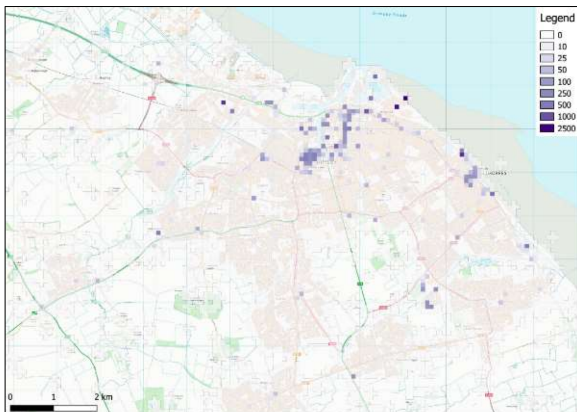
Figure 4-3: Storage cooling demand density map for Grimsby and Cleethorpes and around (units MWh per 100m x 100m square)
